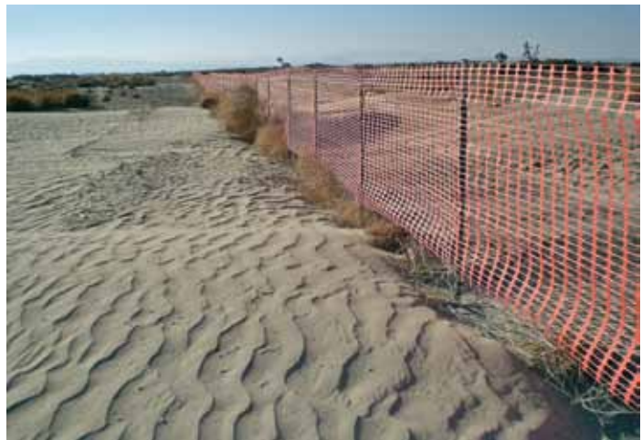
Figure 7: This 50% wind porosity fencing causes sand to deposit on both sides, but more on the downwind side of the fence. (Prevailing wind blows from left to right.)
