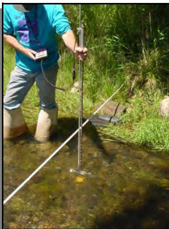
Neal Schaeffer calculates water flow using a Pygmy meter, Digitizer, and measuring tape.
