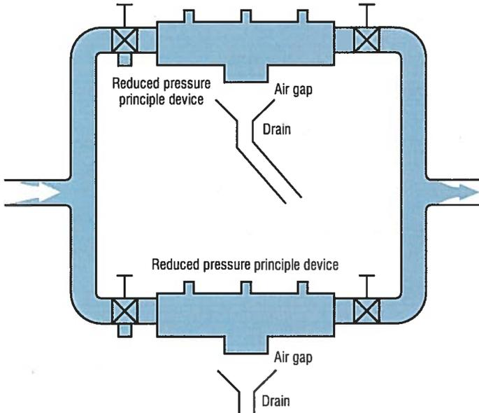
Note: Devices to be set a min. of 12" and a max. of 30" from the floor and 12" from any wall.
