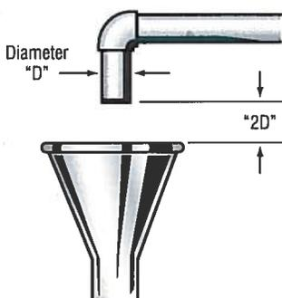
An air gap, although an extremely effective backflow preventer when used to prevent backsiphonage and backpressure conditions, does interrupt the piping flow with corresponding loss of pressure for subsequent use. Consequently, air gaps are primarily used at end of the line service where reservoirs or storage tanks are desired. When contemplating the use of an air gap, some other considerations are:
