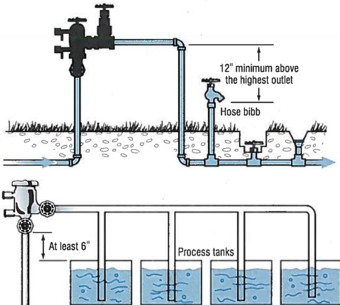
FIGURE 22. Double check valve with atmospheric vent.
