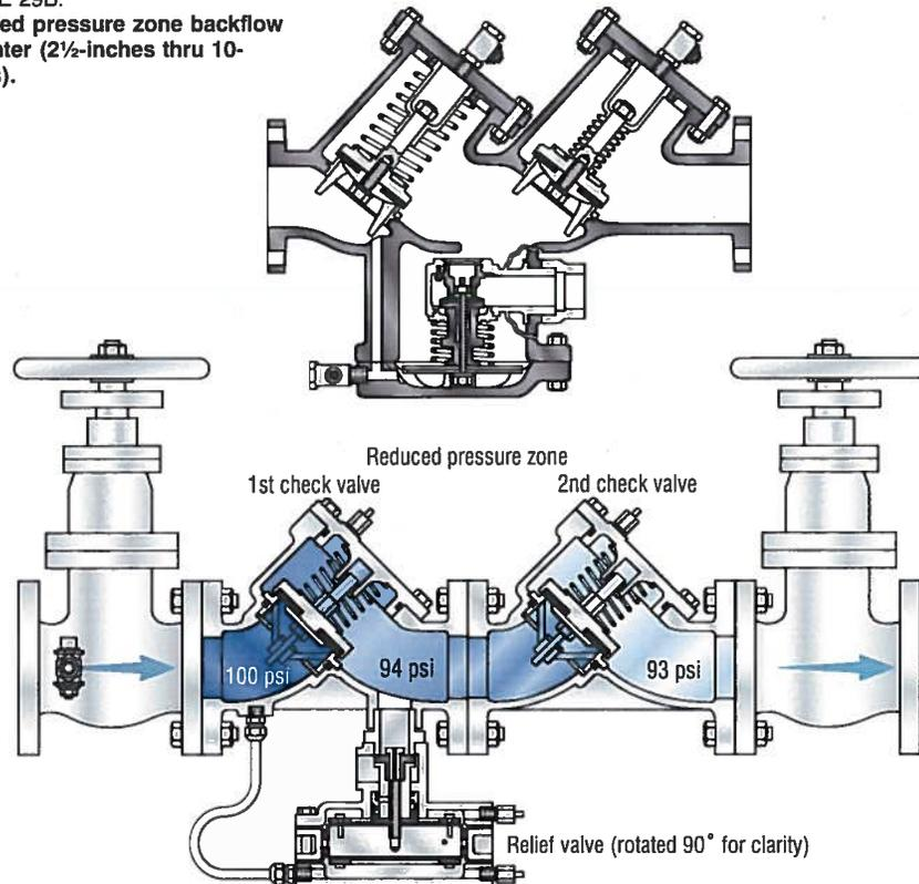
The principles of operation of a reduced pressure principle backflow preventer are as follows:
