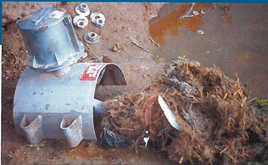
Accurate flow-rate measurements are needed to more efficiently manage nutrients in water from dairy manure ponds, which is later applied during irrigation. Commonly used in agriculture, the propeller meter often becomes entangled with weeds and twine from a dairy manure pond, making it difficult to obtain readings.
